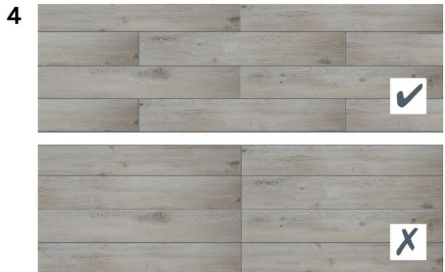
When planning where to start from, ensure that you stagger the joints on each row. There should be at least a 1/3rd of a plank or tile length between each end joint. Do not have all the joints running in a line.
